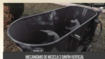
MECANISMO DE MEZCLA 2 SINFIN VERTICAL
