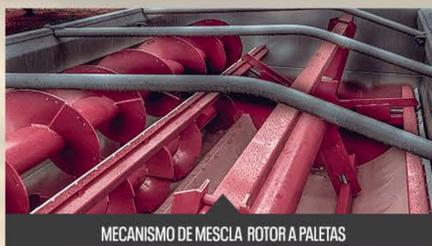
MECANISMO DE MEZCLA ROTOR A PALETAS
