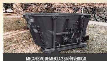
MECANISMO DE MEZCLA 2 SINFIN VERTICAL
